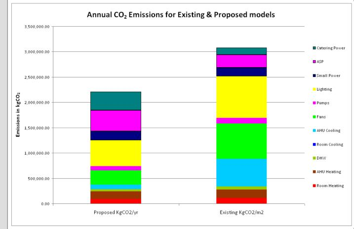
Just looking at the consumption &  $CO_2$  for environmental treatment elements, we can see that total energy consumption has dropped by 46% and  $CO_2$  has dropped by 50%
