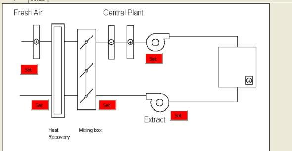
This is a HVAC system where the air enters the zone at a constant volume. The supply air is conditioned in an attempt to meet the heating and cooling demand requirements. If multiple zones are used in the sub-project then the CAV system will meet the demand of the zone that requires the most cooling and then re-heat the other zones.
