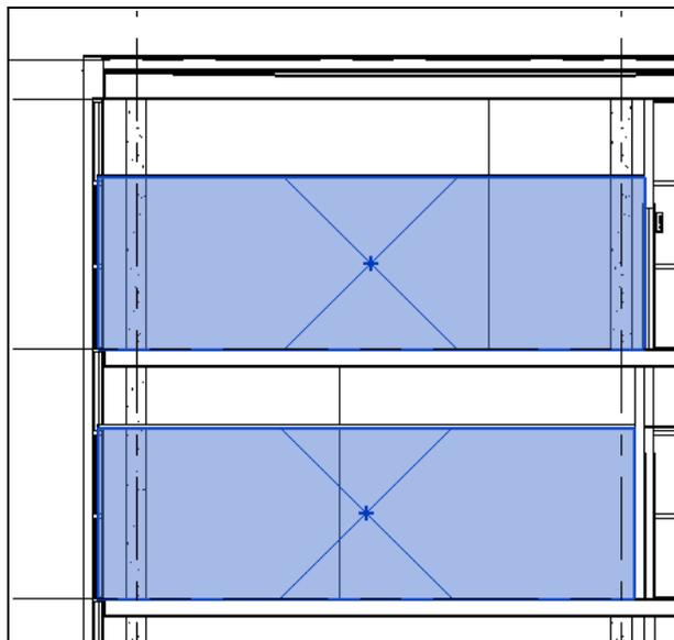
In the section above, two rooms, one directly on top of the other, are separated by a ceiling and a floor with a void between these two elements. If a gbXML was created with the model as it is, the two rooms would not have a link to each other. The solutions are the same as the wall void case:
