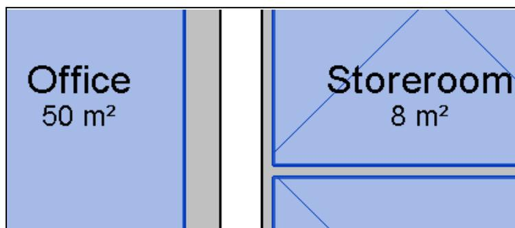
There can be no wall voids that do not contain rooms. As an example, see the picture above – two existing rooms are separated by two walls with a void between them. The geometry would be incorrect if a gbXML was made from this model; the two rooms would have no link and their walls would be marked as the wrong type.
