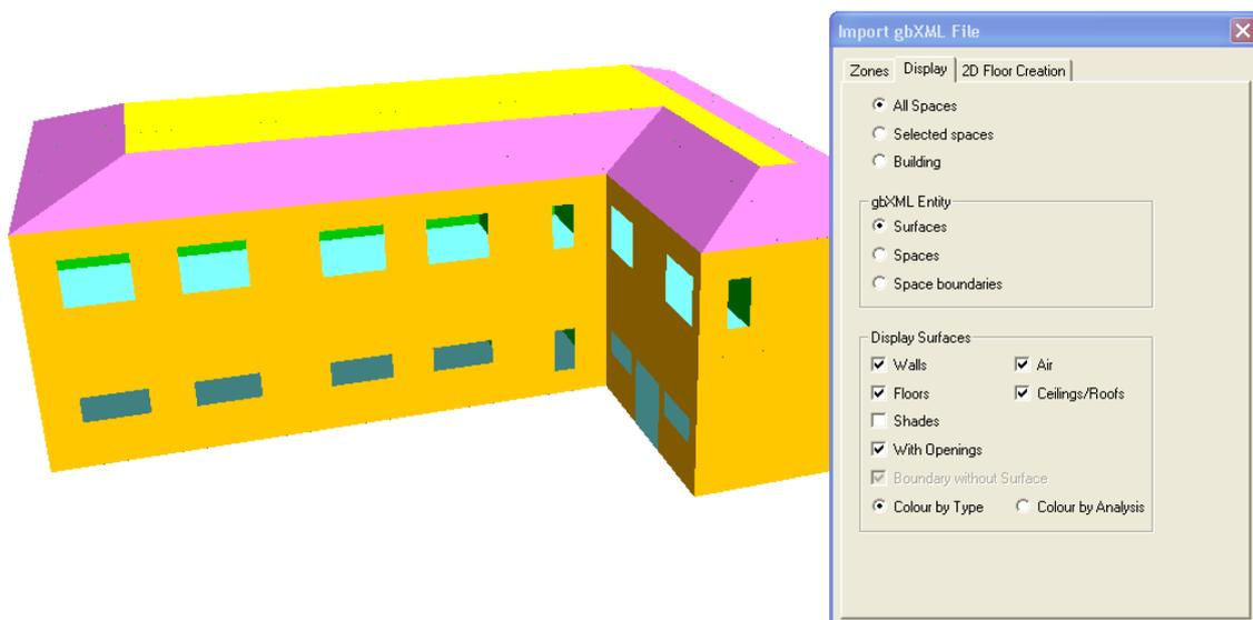
In the image above, hiding the shade surfaces has caused part of the roof to disappear – in this case the issue was that the room limits were set too low and they didn’t reach the top of the roof. In general, if anything disappears which shouldn’t when the shades checkbox is disabled, the solution is to ensure that a room was applied to the area and that the room isn’t prevented from reaching the building surfaces by e.g. a room separation line or badly defined room limit.
