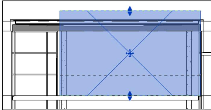
In the section above a room protrudes through the roof. The two most likely causes are that the roof is not room bounding, or that the option “Areas and Volumes” has not been selected in the “Area and Volume Computations” dialog. It is a good idea to select this option before attempting to resolve any room bounding issues, to avoid confusion.
