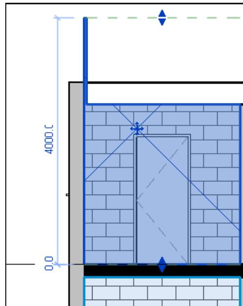
The section above demonstrates that a very small gap in a roof can have a large effect on the room beneath it. The room, highlighted in blue, is leaking out upwards through the gap between the roof and the wall. If this model was exported to a gbXML the room shown would have two large exposed air surfaces.
