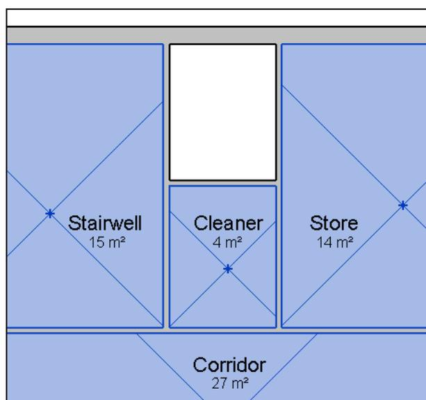
Rooms must be applied to all areas of the building. There should be no region within the shell of the building that is not filled by a room, including risers, ceiling voids, wall voids, floor voids, etc. Any areas not filled by a room will be missing from the gbXML file, and neighbouring walls will be marked as an incorrect type in the gbXML.
