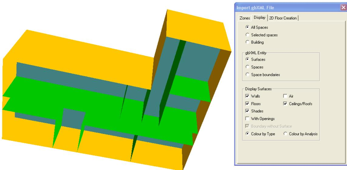
Note that the “With Openings” checkbox is disabled. This option toggles the display of openings on the surfaces (windows, doors and rooflights). The reason for disabling this option is to distinguish between air surfaces that are not displayed due to the fact that they are windows and doors.
