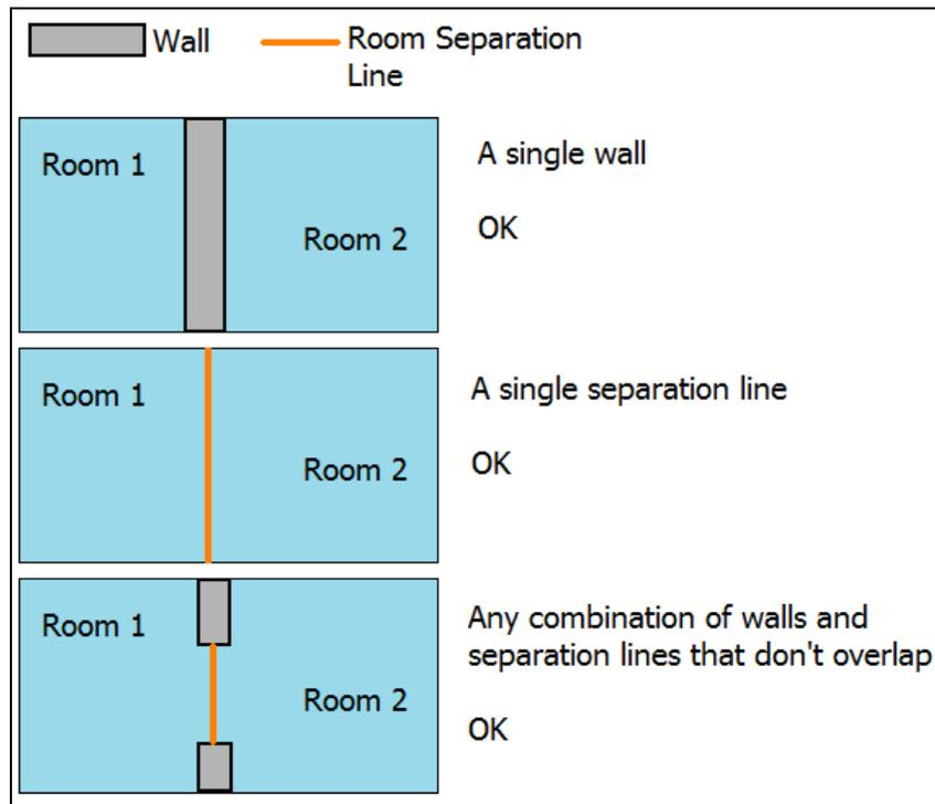
Note that these rules apply equally to links between a room and the outside air, as they do to links between two rooms.
