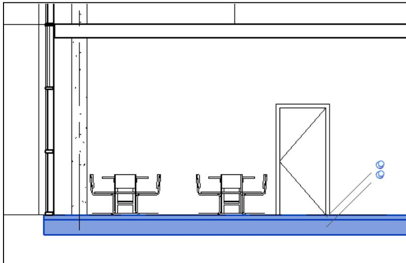
As with walls, there should be no instances where floors and/or ceilings are placed directly in contact with each other. In the case shown by the section above, the room is only considered to be in contact with the uppermost floor element, and the lowest floor element is disregarded. The best solution here is to replace the two floors with a single, thicker element. The quickest solution is to make the top layer non-room-bounding.
