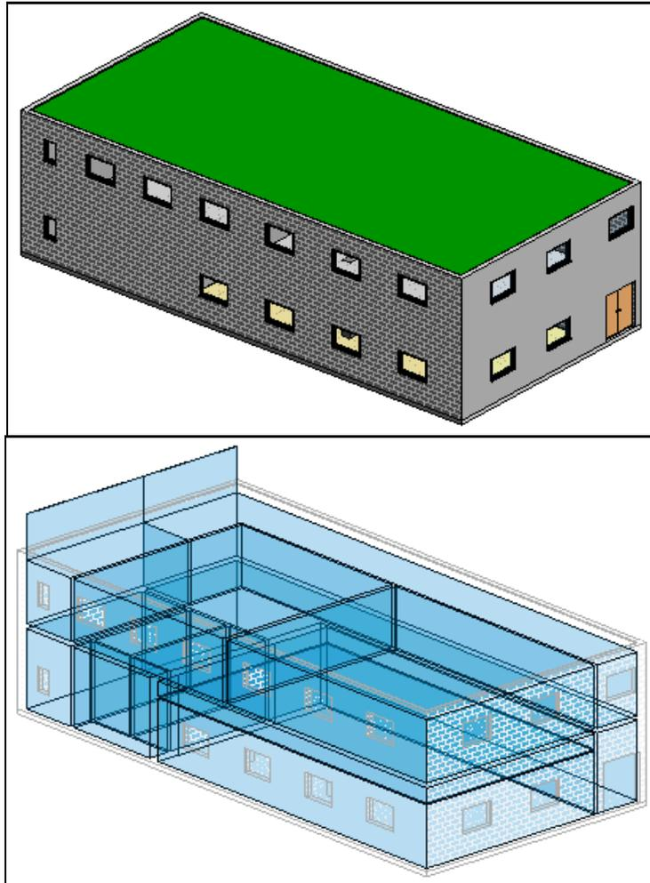
The images above show an example of a building with a gap in its roof. The first image is the building as it appears in the Revit 3D view, and no roof issues are immediately obvious here. The second image shows the building in the Export gbXML dialog. The blue shaded areas are the rooms, and on the left hand side of the image two rooms are sticking out through a thin gap in the roof of the building. The footprint of the roof should be extended to prevent this.
