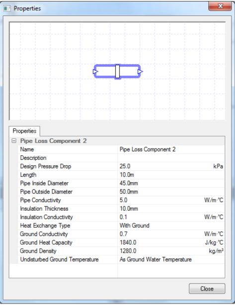
The Pipe Loss Component allows the user to model the heat loss / gain that the fluid will experience when travelling through pipes. The user can model the pipes being placed in the ground or exposed to air. Please note that controllers cannot be used with this component.
