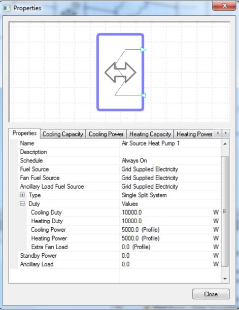
The Air Source Heat Pump component in TAS Systems allows the user to model heat pumps which transfer the load with the air. The two ports on the side of the heat pump, which are light blue, indicate that the air source heat pump can only be connected to refrigerant circuits. Please note that controllers cannot be used with this component.
