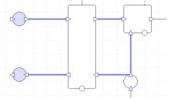
Placing a flow component on these ducts will cause issues with how the air-side economiser works; for instance, the minimum fresh air requirement may not be met.
