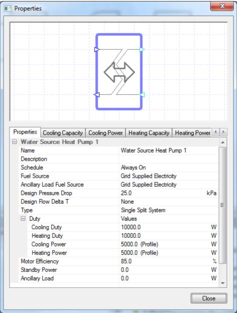
The Water Source Heat Pump component in TAS systems transfers the load from the refrigerant group to the connected fluid circuit loop. Please note that the light blue ports are refrigerant ports and should connect up to the refrigerant group while the dark blue ports are fluid ports and should connect up to the fluid circuit loop. Please note that controllers cannot be used with this component.
