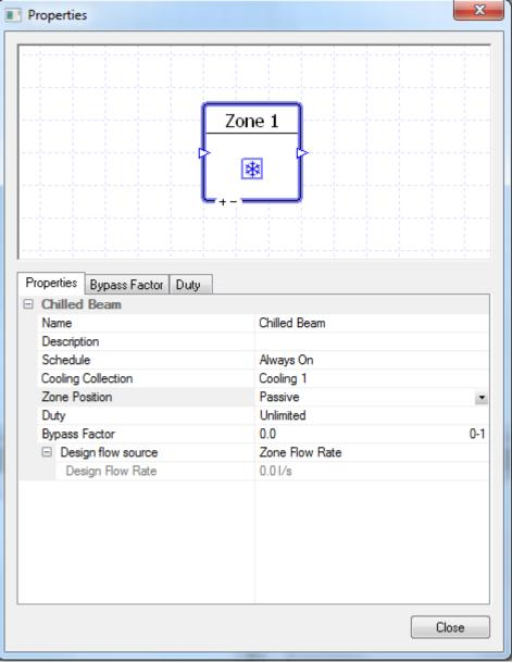
A Chilled Beam component can be used to model an active or passive chilled beam. Cold water is pumped through the beam and cools the surrounding air, which then cools down the space by convection. Please note that the user will need to edit the radiant proportion of the cooling emitter in the zone's internal condition to model the chilled beam correctly. You cannot use controllers with this component and it will always cool the space to the upper limit of the zones thermostat.
